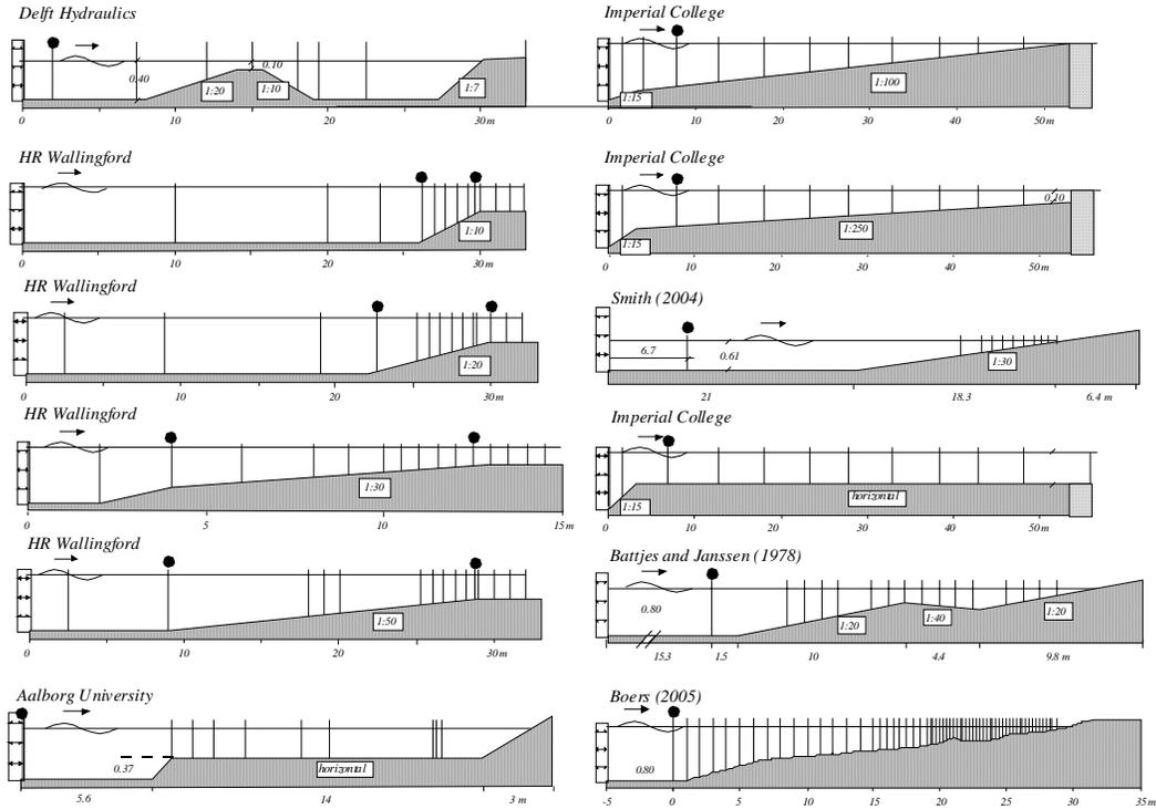
Fig. 2 The configuration of the laboratory observations (calibration and verification). Thin vertical lines indicate wave gauge positions. Solid dots indicate location of incident spectra (wave boundary condition) for the computations.
