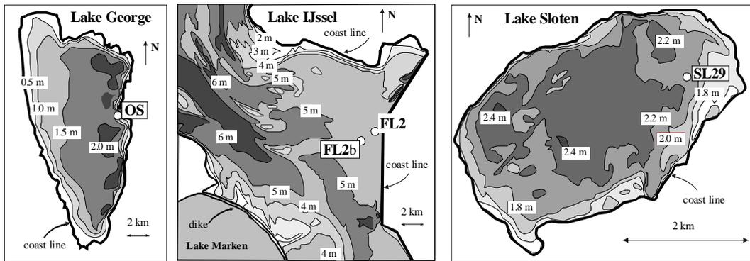
Fig. 3 The bathymetry of the three lakes used for the calibration. The location of observation sites are indicated with OS, FL2, FL2b and SL29.
