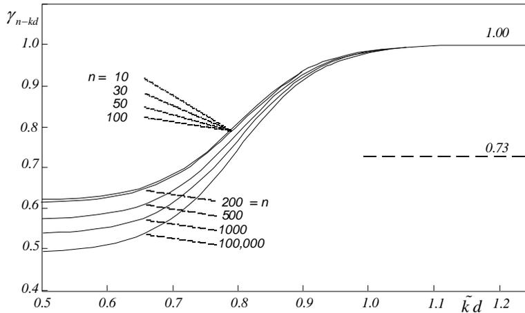
Fig. 1 The calibrated value of  $\gamma_{n-kd}$  as a function of bottom slope  $n$  and normalized depth  $\tilde{k}d$ , with  $\gamma = 0.73$  as reference.
